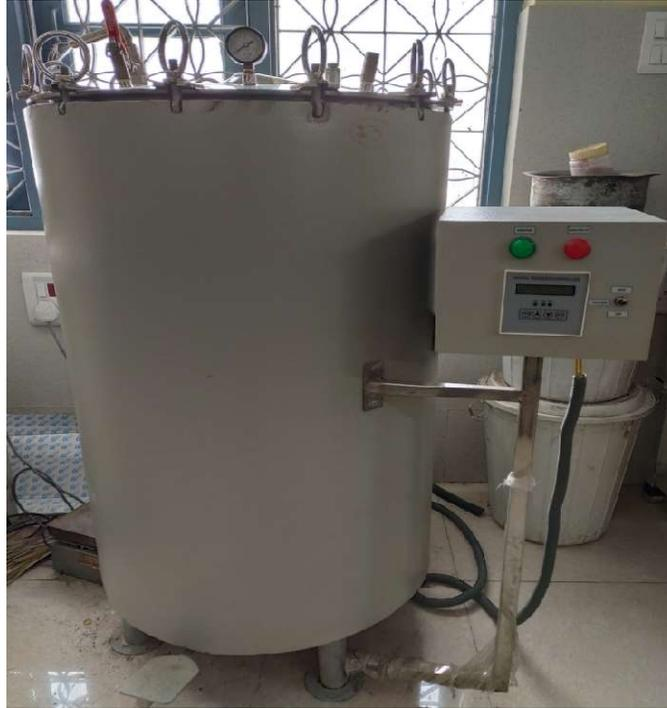
An autoclave is a pressure chamber used to carry out industrial and scientific processes requiring elevated temperature and pressure in relation to ambient.
