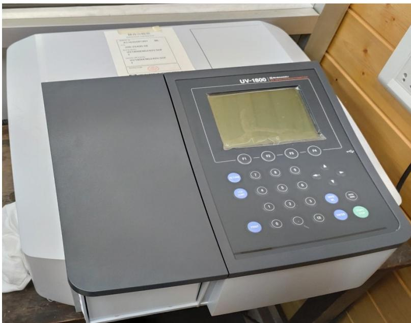
Ultraviolet-visible spectroscopy or ultraviolet-visible spectrophotometry (UV-Vis or UV/Vis) refers to absorption spectroscopy or reflectance spectroscopy in part of the ultraviolet and the full, adjacent visible spectral regions.
