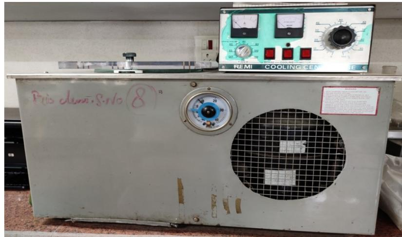
A centrifuge is a device for separating particles from a solution according to their size, shape, density viscosity of the medium and rotor speed. Refrigerated laboratory centrifuges temperature ranges as wide as  $-20^{\circ}\text{C}$  –  $40^{\circ}\text{C}$ , making them perfect for DNA, RNA, PCR or antibody analysis.
