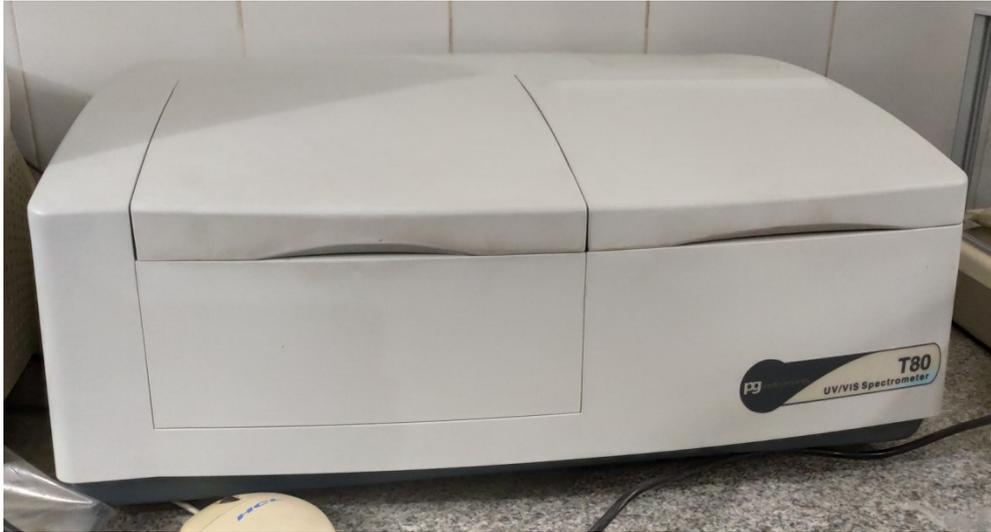
Ultraviolet–visible spectroscopy or ultraviolet–visible spectrophotometry (UV–Vis or UV/Vis) refers to absorption spectroscopy or reflectance spectroscopy in part of the ultraviolet and the full, adjacent visible spectral regions.
