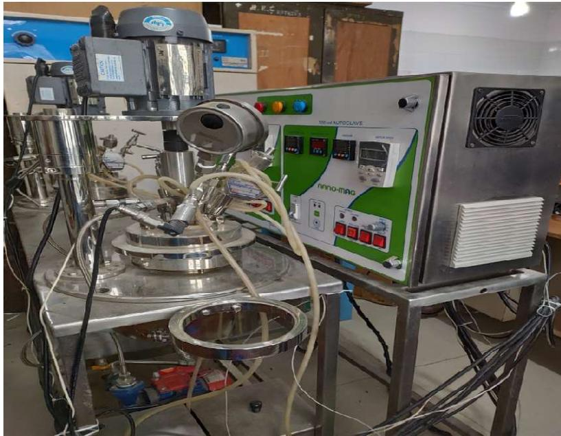
An autoclave is a pressure chamber used to carry out industrial and scientific processes requiring elevated temperature and pressure in relation to ambient.
