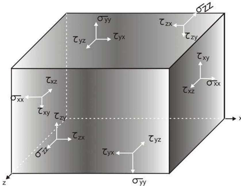
Figure 2.6. Stress on an infinitesimal element .
