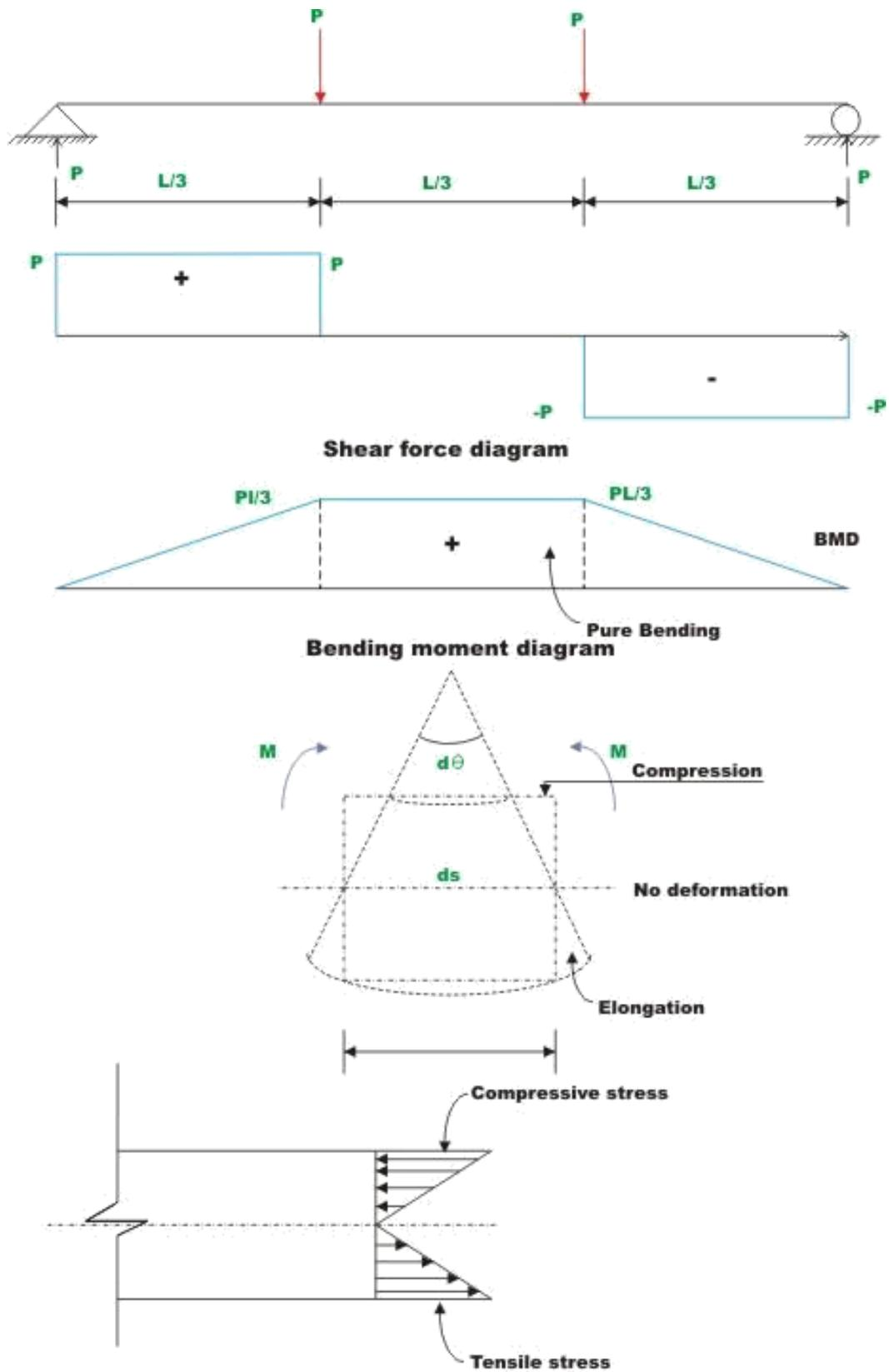
**Fig. 2.9 BENDING DEFORMATION**
