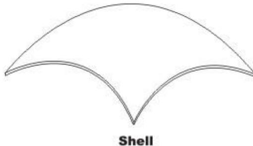
**Fig 1.1(b) Commonly Used Structural Forms**
