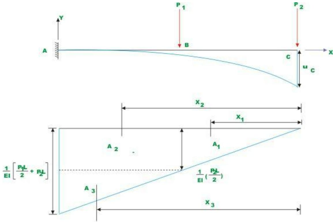
**Fig 2.1 Cantilever Beam with Two Concentrated Loads**
