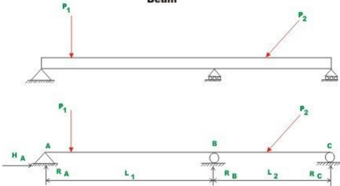
**Fig 1.7 Statically Indeterminate Beam**
