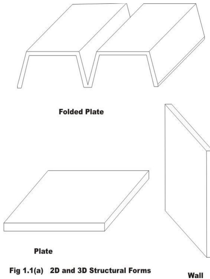
**Fig 1.1(a) 2D and 3D Structural Forms**
