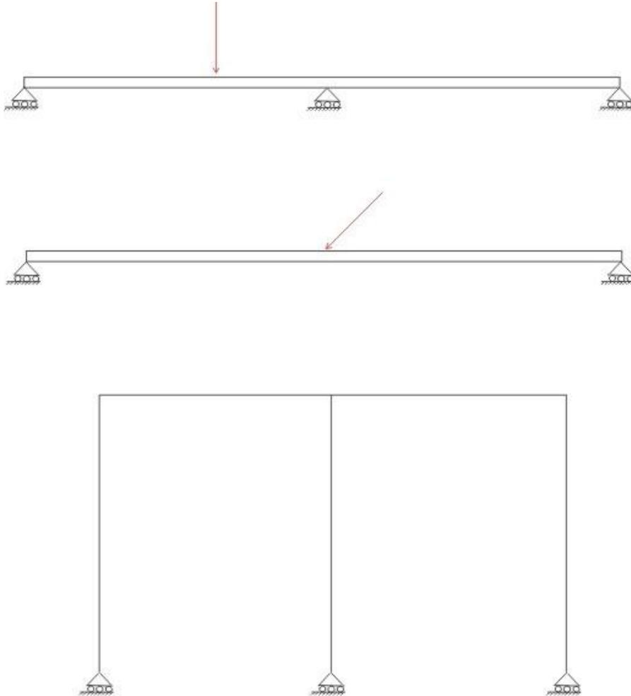
**Fig 1.14 Kinematically Unstable Structures**
