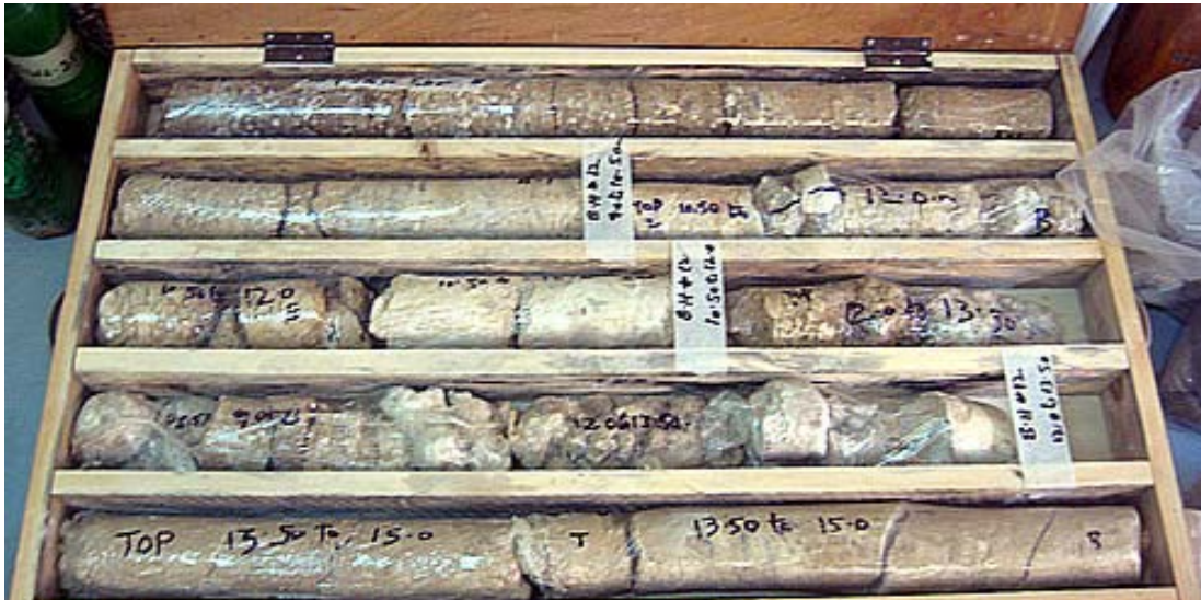
Figure 2.2: Picture showing core box with cylindrical cores as recovered
