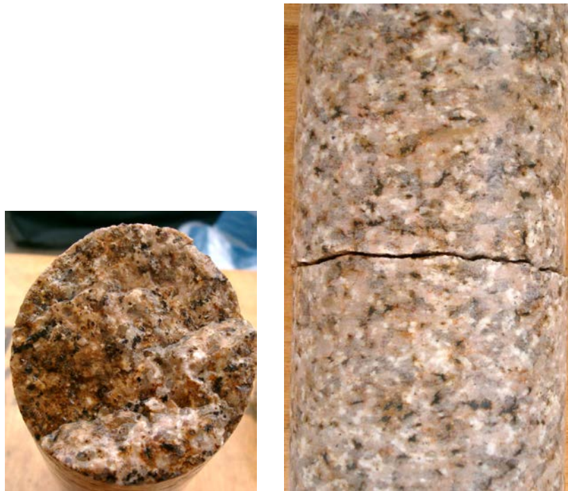
Figure 2.3: Drilling induced fractures
