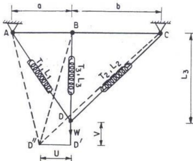
The horizontal ( $U$ ) and the vertical ( $V$ ) displacements of the point D is calculated as follows
