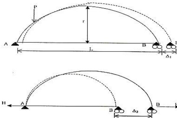
**Theory:** - The two hinged arch is a statically indeterminate structure of the first degree. The horizontal thrust is the redundant reaction and is obtained by the use of strain energy methods. Two hinged arch is made determinate by treating it as a simply supported curved beam and horizontal thrust as a redundant reaction. The arch spreads
