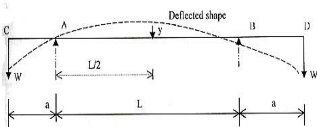
**Theory:** - For the beam with two equal overhangs and subjected to two concentrated loads W each at free ends, maximum deflection y at the centre is given by central upward deflection. Central upward deflection,  $y = W.a.L^2 / 8EI$
