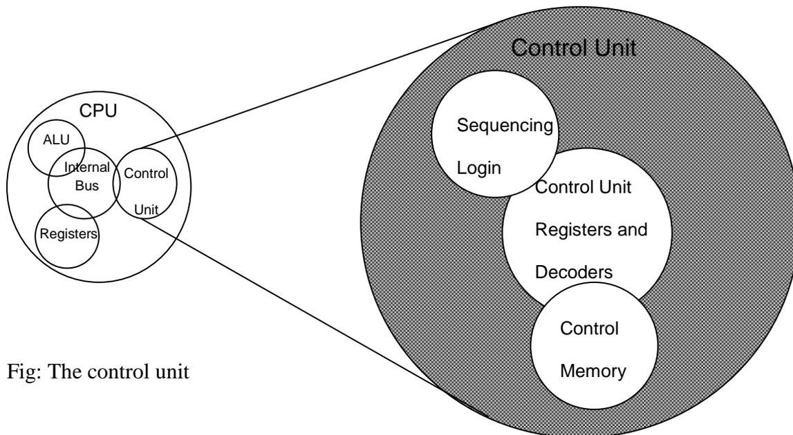
Fig: The control unit
