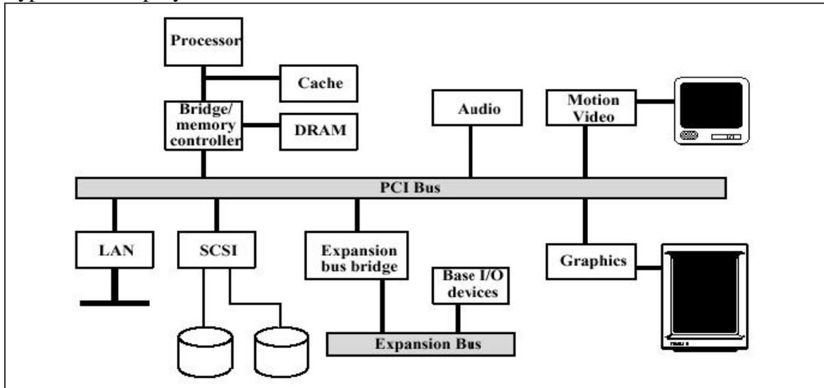
Note: Bridge acts as a data buffer so that the speed of the PCI bus may differ from that of the processor's I/O capability.
