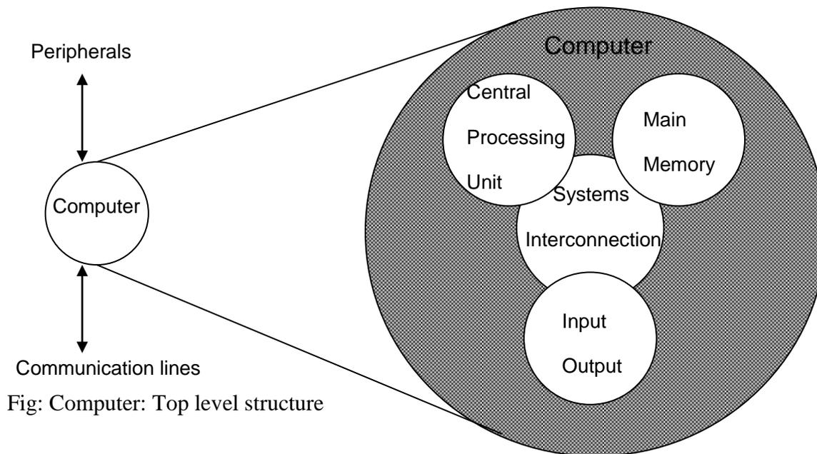
Fig: Computer: Top level structure
