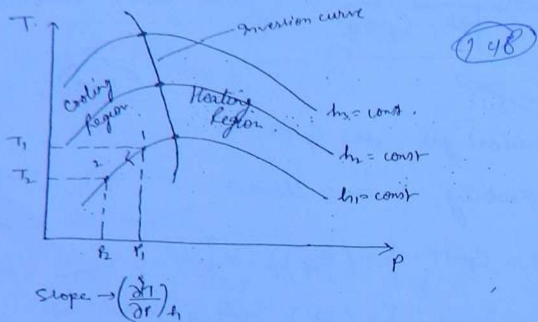
$$\mu = \left(\frac{\partial T}{\partial P}\right)_h = \text{slope of isenthalpic curves on T-P diagram.}$$
