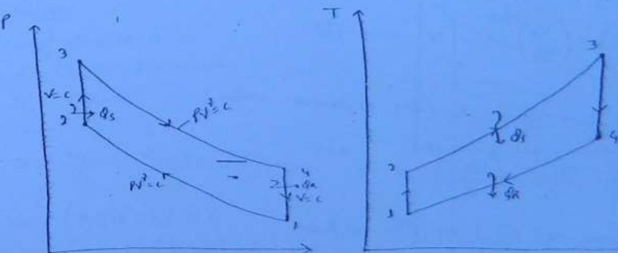
$$\left. \begin{array}{l} p_1 V_1^{\gamma} = p_2 V_2^{\gamma} \\ \frac{V_1}{T_1} = \frac{V_2}{T_2} \end{array} \right\} \left( \frac{p_1}{p_2} \right)^{\frac{1}{\gamma}} = \frac{T_2}{T_1}$$
