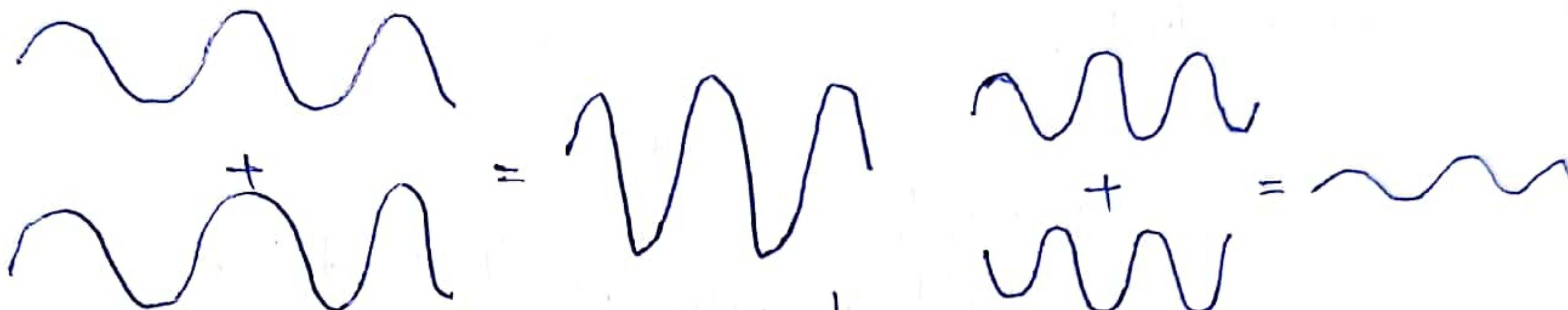
In constructive interference, superposed waves in phase reinforce each other.
