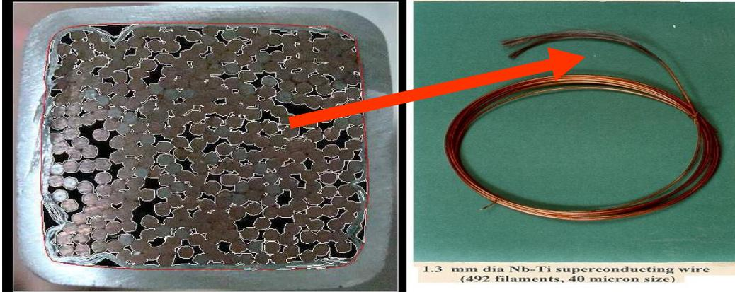
Cross section of 20x20mm CICC containing 336 wires of 0.8mm dia out of which 48 nos. are SC wires
