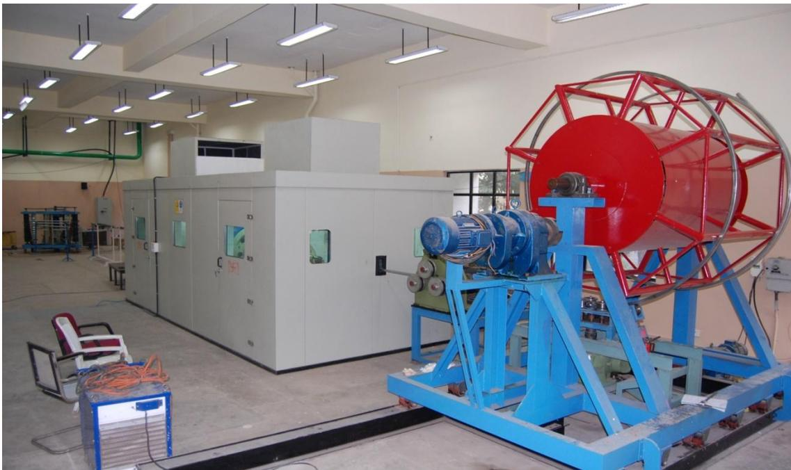
**Fig: On-line CICC Fabrication Facility developed at AFD, BARC**
