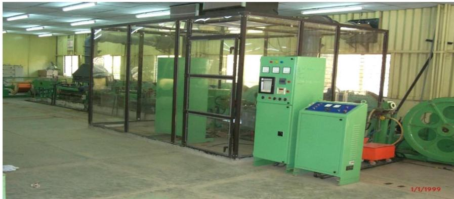
Continuous soldering unit for superconductor wire
