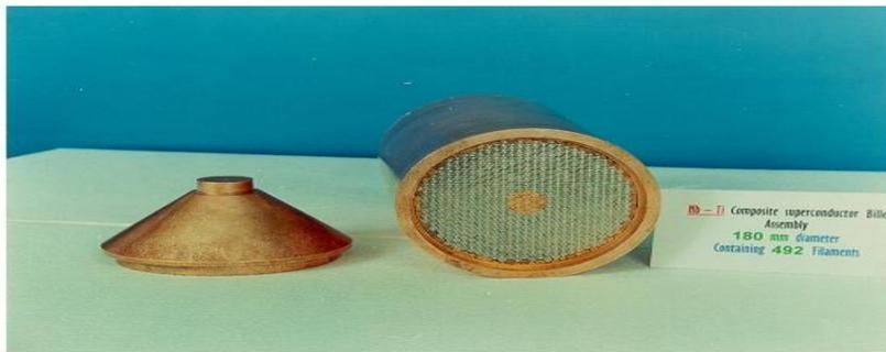
**Nb-Ti multi filamentary billet assembly developed at AFD, BARC.**
