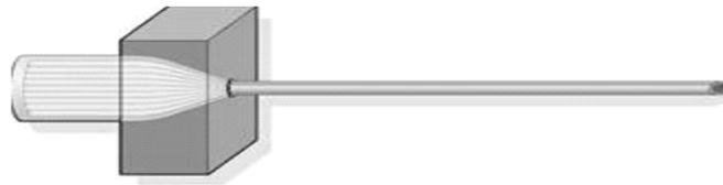
Fig. Showing extrusion of superconducting billet
