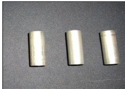
Fig. 2 Shows wear test specimen
