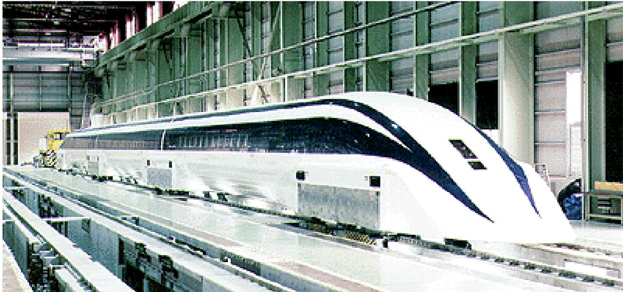
Fig. Maglev test vehicle, 552 km/hr
