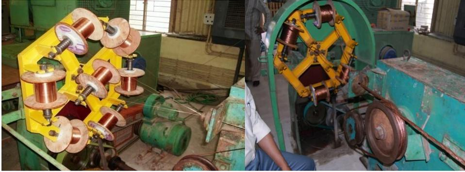
Final Stage Cable Containing 504 wires of 0.8mm dia
