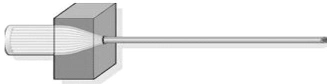
Fig. Showing extrusion of superconducting billet
